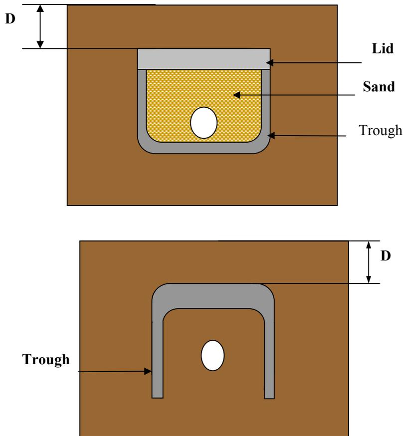
**Figure 6C - Explanation of the Depth of the Direct Burial System**
