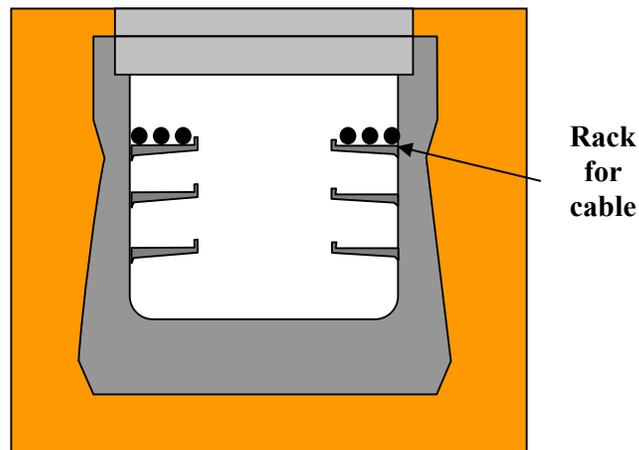
**Figure 6B - Example of Draw-in Culvert System**
