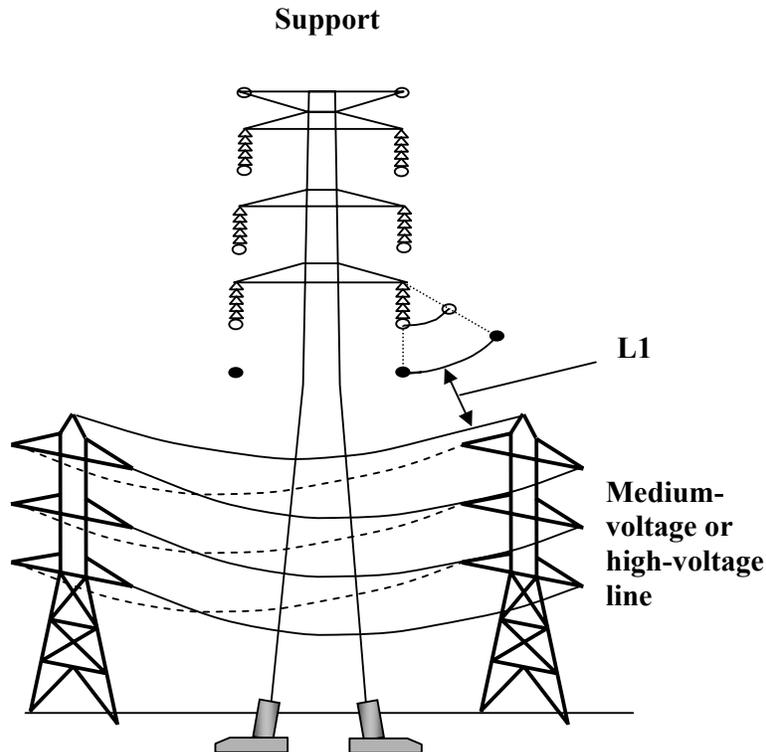
**Figure 10 - Proximity and Crossing with Medium-voltage Lines and High-voltage Lines**
