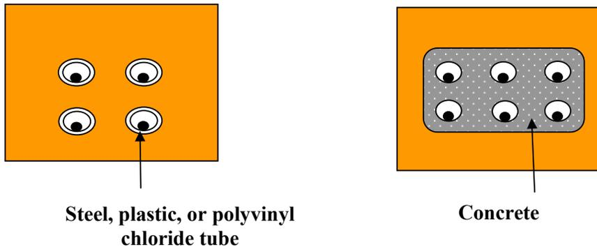
**Figure 6A - Example of Draw-in Conduit System**
