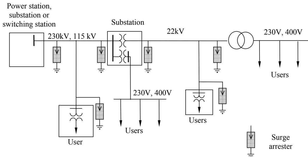
**Figure 11 - Installation Points for Surge Arresters**
