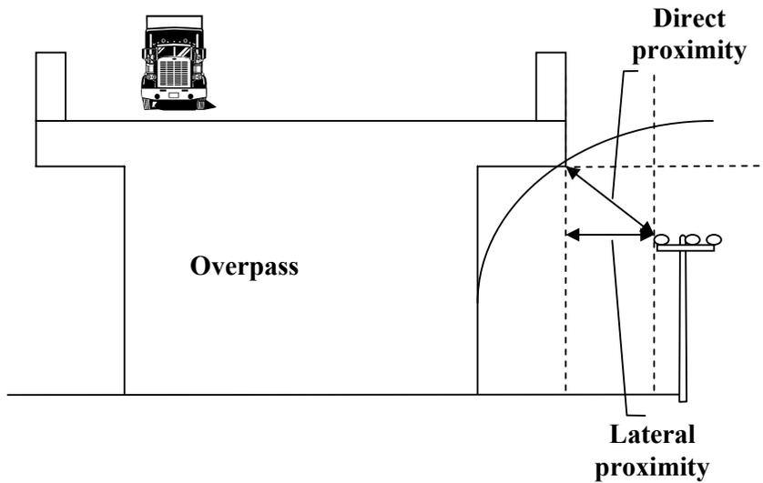
**Figure 13 - Explanation of Direct Proximity and Lateral Proximity (Overpass)**
